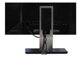
After attaching all necessary cables to your monitor and computer, (See <u>Connecting Your Monitor</u> for cable attachment,) use the cable management slot to neatly organize all cables as shown above.
